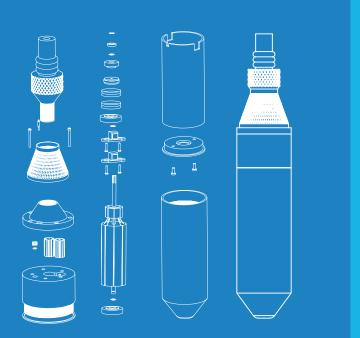
Diameter: 1.75" Length: 9.16" Weight: 2.5 lbs. Materials: 304 Stainless Steel Teflon® Rotors Viton Housing seal Carbon motor seal
